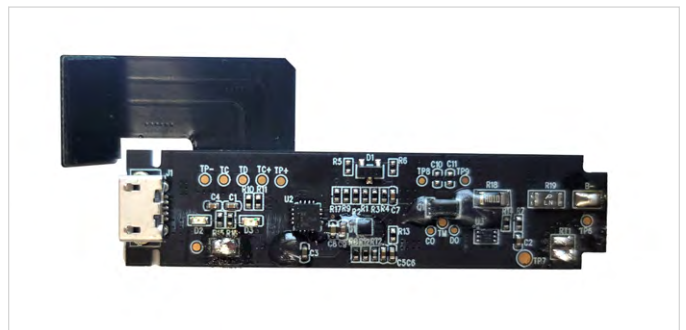
Figure 10: Ring Battery Pack BMS
